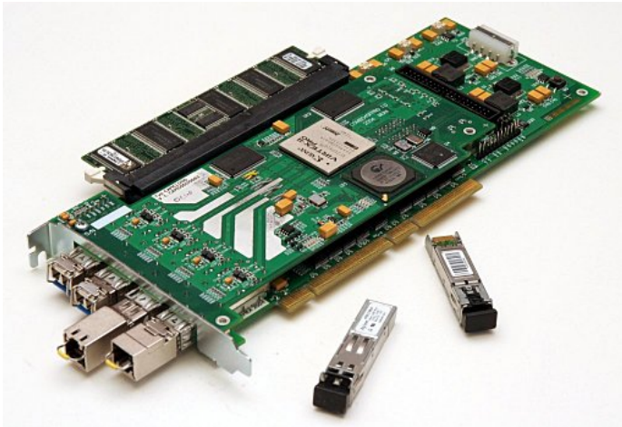
Fig. 2. FlowMon - COMBO6X PCI-X 64/66MHz hardware accelerated card [14]
